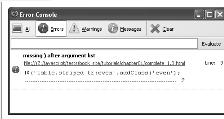
Figure 1-6: Firefox's JavaScript console identifies errors in your programs. The console keeps a list of errors for previous pages as well, so pretty soon the list can get very long. Just click the Clear button to erase all the errors listed in the console.
