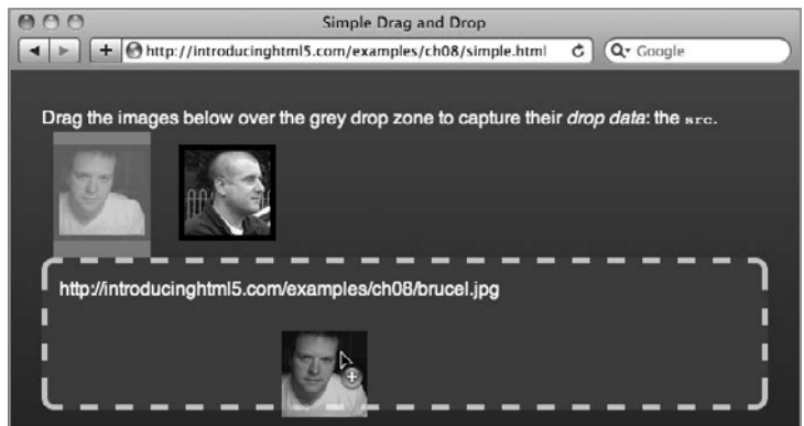
FIGURE 8.1 All images and links are draggable by default. With a little more code, you can make them droppable too.
