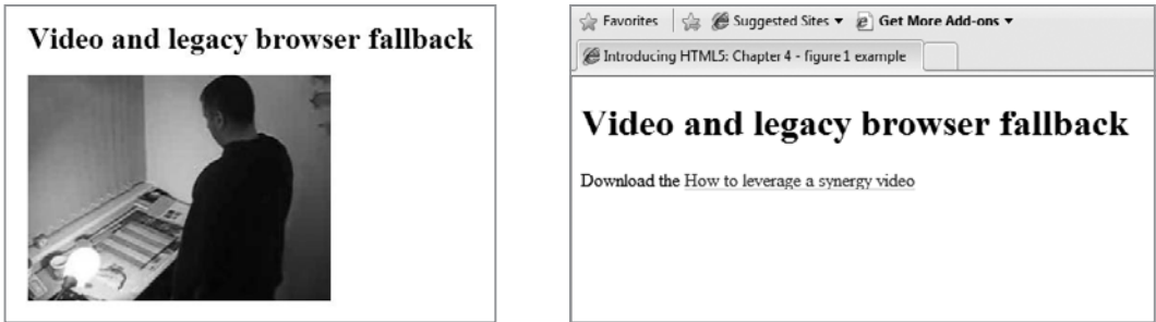
FIGURE 4.1 HTML5 video in a modern browser and fallback content in a legacy browser.
