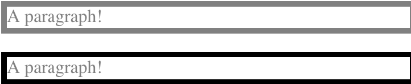
Figure 8-26. Border colors based on the element’s foreground and the value of the border-color property
