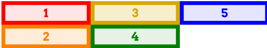
Figure 13-45. Column-oriented grid flow
