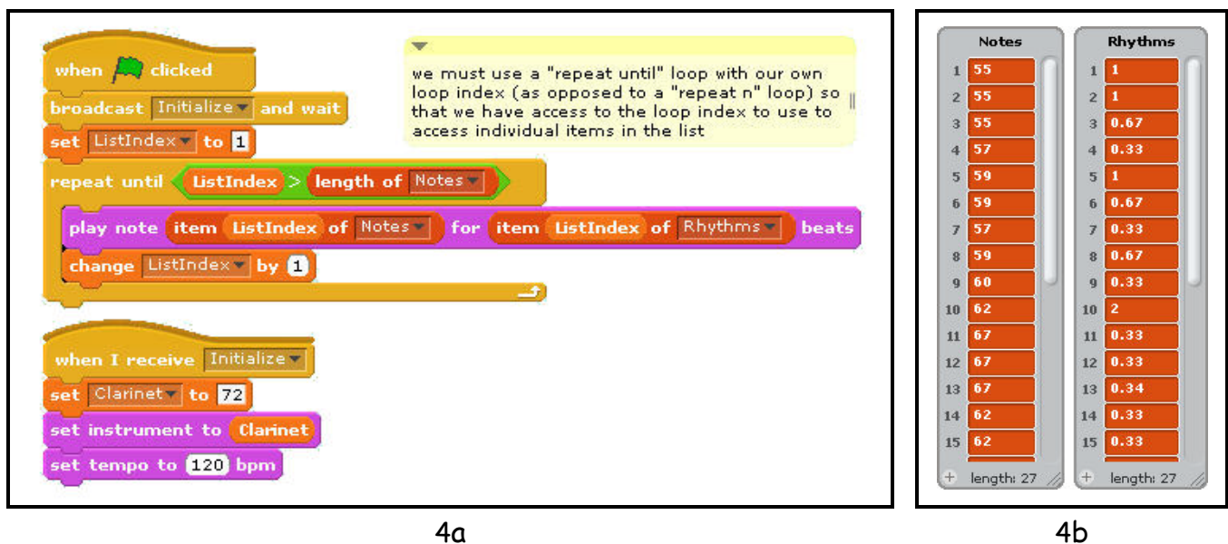
Figure 4. Processing Scratch lists of notes and rhythms for Row, Row, Row Your Boat. [5]
