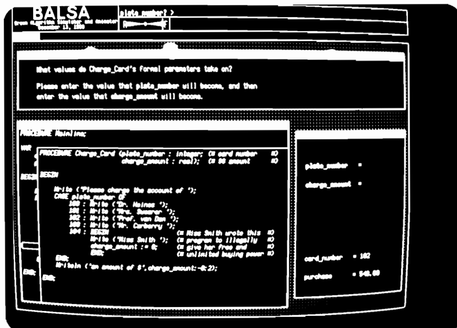
Figure 8. Overlaid code of called procedure and appearance of formal parameters in adjacent window.
