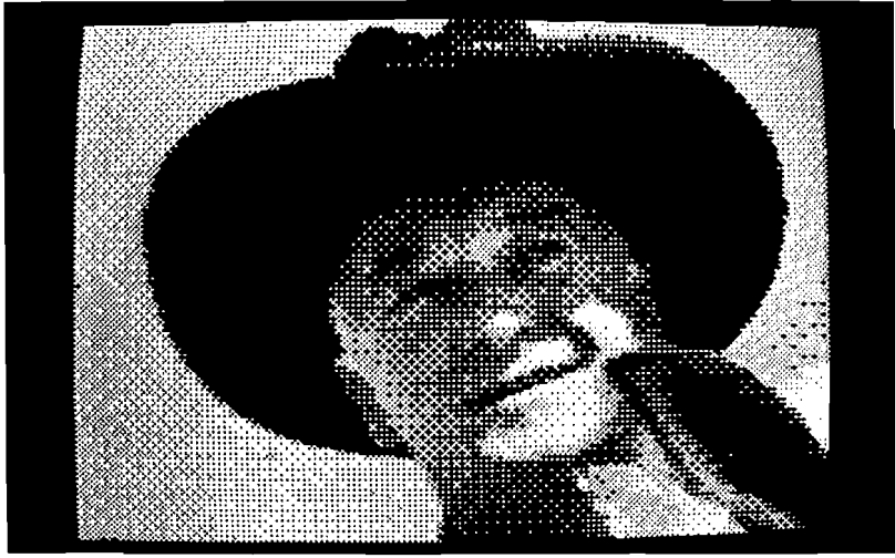
FIGURE 6-8. A Complex Display that Can Best Be Stored in Bit Map Form.
